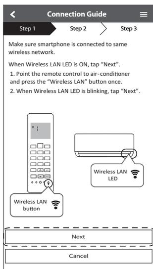
1. Ensure Wireless LAN LED is ON. point the remote control to air conditioner and press Wireless LAN
